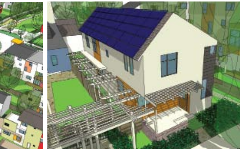
Geos, a 250-home, urban mixed-use neighborhood in Arvada, Colorado, is expected to be the largest net zero-energy solar community in the United States. To maximize solar access within a traditional neighborhood layout, alternative single-family houses are set back on an alley to allow maximum solar access for each house.
